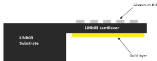
Figure 4.4.1 Cantilever with Aluminum IDTs on the top layer and gold layer on the bottom one
